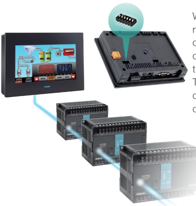
With RS-422/RS-485 communication networks, termination resistors are often required to improve the reliability of communications. External termination resistors can make communication wiring onsite complex. To solve this problem, the P5 provides built-in termination resistor switches. Terminating can be achieved by turning on the switch to connect to termination resistors, or turn off the switch to disconnect the resistors.
